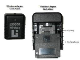
2. Slip the wireless adapter over the DAS module until it clicks into place.
